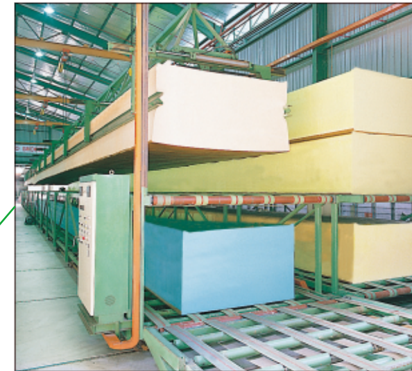
Block Storage System with crane unit
